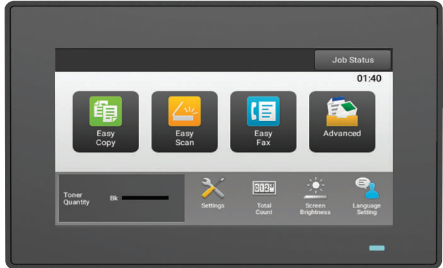
4.3" (diagonally measured) customizable touchscreen display.
